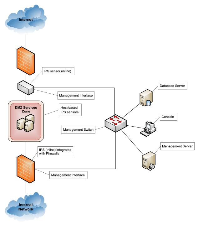
Figure 2 - Deployment example - gateway perimeter
